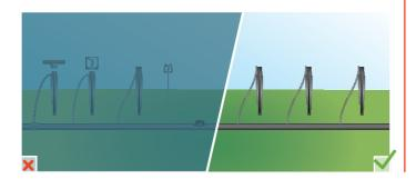
Don't put too many emitters (insufficient water will come out) or too few (will result in high pressure and wasted water) on one line.
